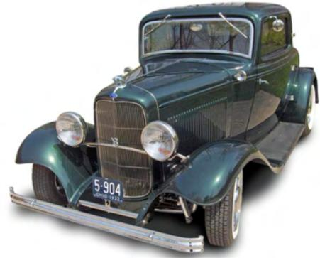
Want a “new” 32 Ford? Check out Brookville Roadster, makers of replica steel 1932 Ford roadster and three-window coupe bodies. Brookville uses period stamping machines to create panels that are interchangeable with stock Ford components. The company will sell a complete body and, if you want, it will assemble a roadster or a coupe on a re-pop chassis
